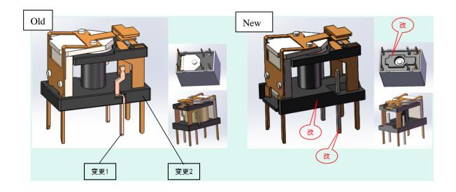
Change 1: Change coil pins' shape and structure Change 2: Change bobbin' shape and structure
